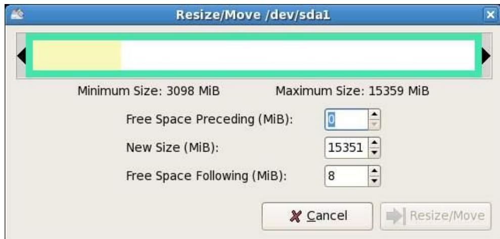
Change the *New Size* field to 8000 MiB and click on the *Resize/Move* button at the bottom of the dialog. The Resize action will then appear in the *Pending* panel at the bottom of the main GParted screen and the new space will be displayed in the graphical representation of the disk as *Unallocated space*:
