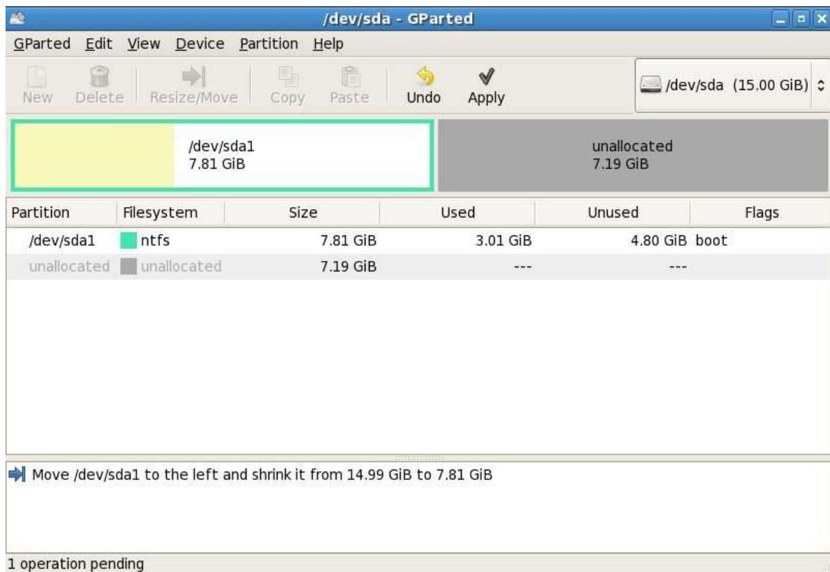
To commit the resize click on the *Apply* button in the toolbar and confirm the resize in the subsequent warning dialog. The *Apply pending operation* dialog will appear and display the progress of the resize. Once the resize is completed successfully, close the dialog and exit *GParted*.
