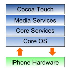
Some diagrams designed to graphically depict the iOS software stack show an additional box positioned above the Cocoa Touch layer to indicate the applications running on the device. In the above diagram we have not done so since this would suggest that the only interface available to the app is Cocoa Touch. In practice, an app can directly call down to any of the layers of the stack to perform tasks on the physical device.
